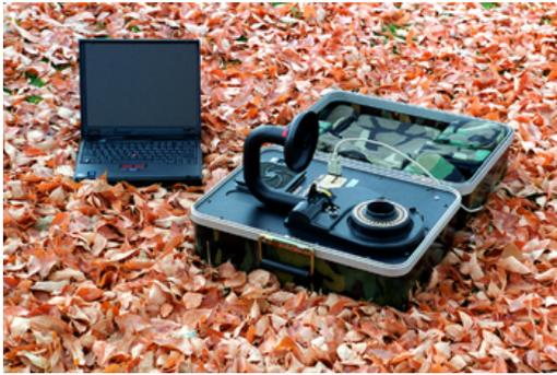
Figure 1. Field portable real-time PCR instrument
